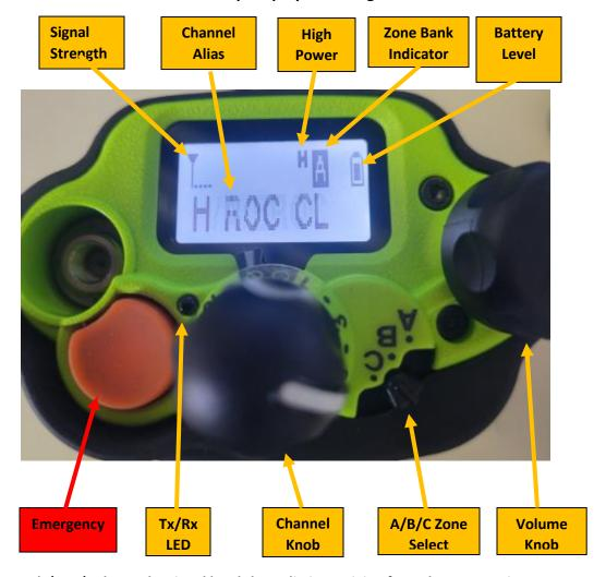
Signal Strength (RSSI): Shows the signal level the radio is receiving from the current site.
