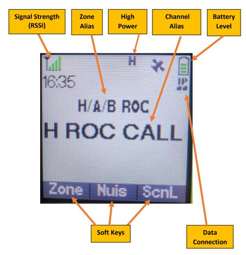
Signal Strength (RSSI): Shows the signal level the radio is receiving from the current site.
