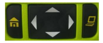
Home Button: Used to return the radio from a menu/configuration mode.
